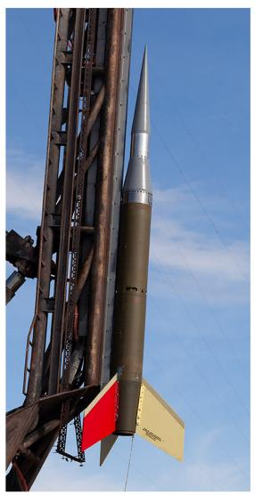
The Improved Orion is a single stage, unguided, fin stabilized rocket system which uses a surplus Army rocket motor having a dual phase propellant. Three fins provide forces for rolling up the vehicle in flight for stability.
